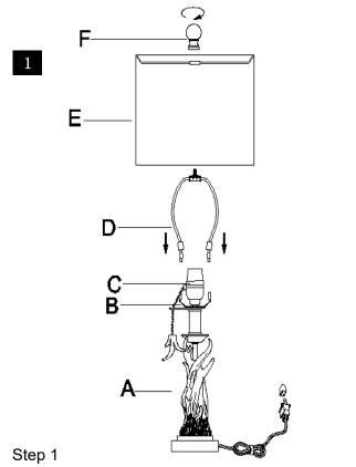
Insert the Harp (D) into the Saddle (B). Put the shade(E) on the Harp(D), then tighten the Finial (F)into the Harp (D)
