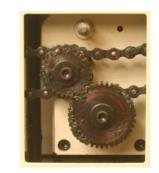
Behind the cover on the left is the feed rate gear set. Swapping these gears on their shafts changes the feed rate from 10 FPM to 20 FPM as shown on the diagram on the cover.
