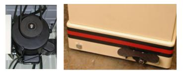
The 1 ½ HP motor (left) has plenty of power for planing and molding operations. Wheels built into the base cabinet (right) make moving the machine easy. The pedal locks and unlocks the wheels.
