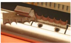
Installing molding knives 2"-long and under does not require removing the planing knives or the outboard gib bars. The spacers seen here are replaced with the molding knife and the same short gib bar is used to secure it.
