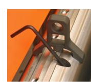
The straight planing knives are retained with gib bars, broken into three segments to accommodate the molding knives. A jack screw under each end of the planing knives and this easy to use knife height gauge make setting this machine up fast and simple.
