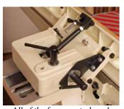
All of the fence controls and adjustments are grouped near the center for easy access.
