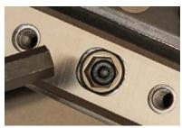
The 3-knife cutterhead in the JJ-6CSDX (left) features our exclusive quick-set system that uses a cam (right) at each end of the knife to make adjustments. Once set, the knives can be reversed or replaced without having to go through the adjustment procedure again!
