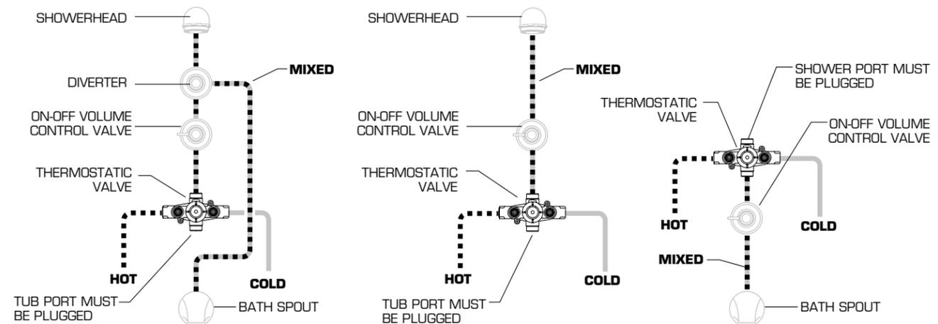
**IMPORTANT:** WHEN USING THIS VALVE AS A BATH/SHOWER, A SEPARATE DIVERTER AND ON-OFF VOLUME CONTROL VALVE IS REQUIRED FOR PROPER OPERATION.
