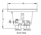
Note: Drain installation is non-standard, vertical overflow connection requires offset.
