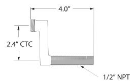
Arm for use with wall mounting. Not needed for freestanding supply lines.
