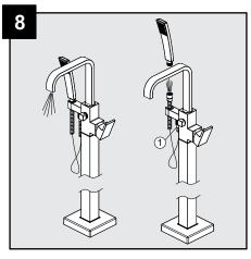
Connect the flexible supply lines (1) to the water supplies (2).
