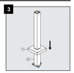
Place the escutcheon (1) over the standpipe (2) and then push it to the base.
