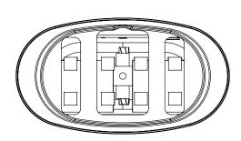
Centerset faucet mounting area - MU66000 Low-profile Overflow Kit required for installation\*
