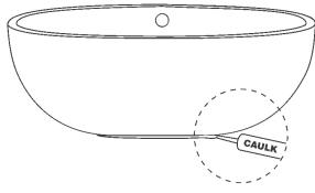
Carefully set tub into position (Figure 7) and connect the drain harware (previously installed).
