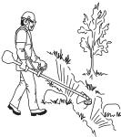
Keep a good balance and a firm foothold. Do not overreach. Keep proper footing and balance at all times. 6 Always hold the machine with both hands. Hold the machine on the right side of your body. Keep all parts of your body away from the hot surfaces. Keep all parts of your body away from the rotating cutting attachment.
