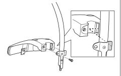
• Fit the dust cup on the shaft. The nut must be completely covered by the dust cup.
