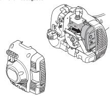
In countries that have a warm and dry climate there is a significant risk of fire. We therefore fit certain mufflers with a spark arrestor screen. Check whether the muffler on your machine is fitted with this kind of screen.
