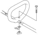
• Fit the bolt, securing plate and wing nut as shown in the diagram. Tighten the wing nut.
