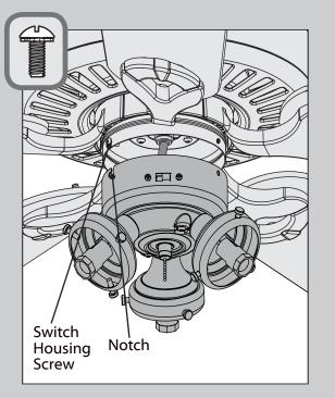
Partially install two of the switch housing screws found in the ≡ hardware bag. Align the notches in the sides of the lower switch housing with the screws on the upper switch housing. Twist the lower switch housing clockwise to lock into place.
