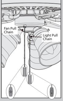
The fan pull chain controls the speed: high, medium, low, and off.
