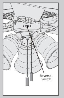
To switch the direction of air flow, move the reverse switch to the opposite position.
