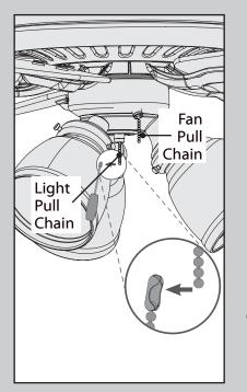
Connect the appropriate pull chain pendant to each of the short chains coming from the switch housing.
