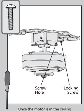
Solution in the two locking screws found in the ★ hardware bag to secure the motor to the ceiling bracket.
