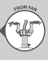
CONNECT WIRES FROM RECEIVER TO FAN - Using the blue wire connectors connect the white wire from the receiver (marked "common out") to the white wire from fan. Connect the black wire from the receiver (marked "fan out") to the black wire from the fan. Connect the blue wire from the receiver (marked "light out") to the blue wire (or possibly black with white stripe) from the fan.
