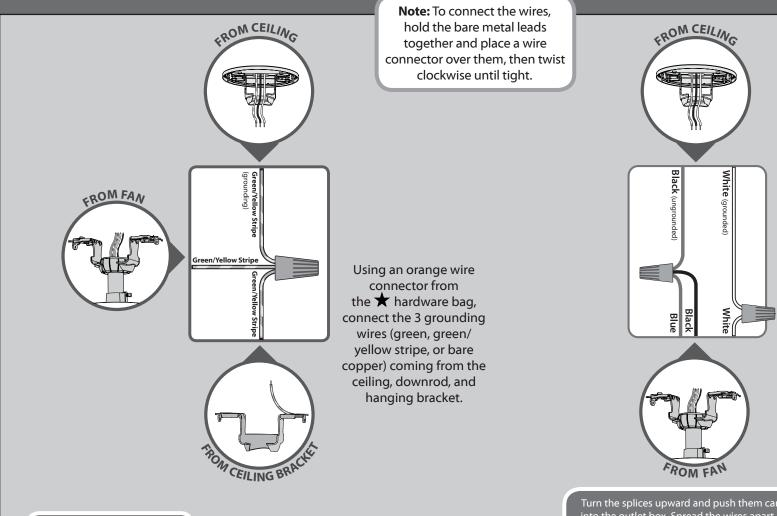
Using the orange wire connectors from the  $\bigstar$  hardware bag, connect the black wire (ungrounded) from the ceiling to the black and the blue wires from the fan. Connect the white wire (grounded) from the ceiling to the white wire from the fan.
