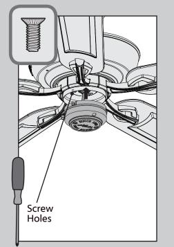
► Lift the lower switch housing until the screw holes are aligned with the screw holes in the upper switch housing. Install the three switch housing screws found in the = hardware bag.
