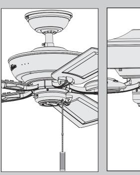
The pull chain controls the fan: from high to off. **Changing the direction of air flow** - move the reverse switch to the opposite position.
