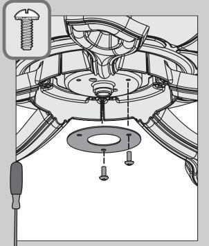
Align the screw holes in the switch
