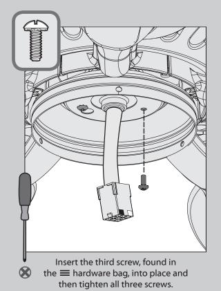
Make sure the upper switch housing is securely attached to the mounting plate. Failure to properly secure all 3 assembly screws could result in the switch housing fixture falling.
