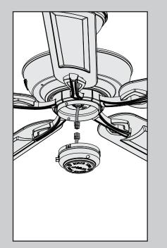
Connect the plugs from the upper and lower switch housings. Make sure to line up the colored markings on the plug connectors.
