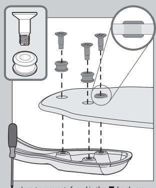
Insert grommets found in the **I** hardware bag into the holes in the blades, then secure each blade to a blade iron with screws found in the **A** hardware bag.
