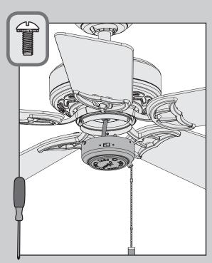
Partially install two of the switch housing screws found in the hardware bag. Align the notches in the sides of the switch housing with the screws on the upper switch housing. Twist the lower switch housing clockwise to lock into place. Install the third switch housing screw. Tighten all three screws.
