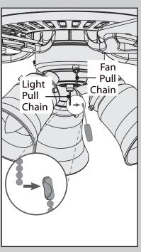
Connect the appropriate pull chain pendant to each of the short chains coming from the switch housing.
