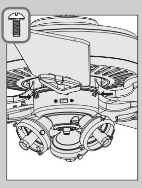
Install the third switch housing screw.
