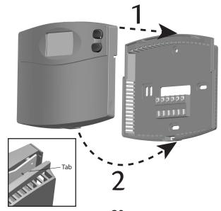
4. Place the top of the thermostat over the two tabs on the wall plate. Press the thermostat onto the wall plate and press to snap the bottom tab into place.
