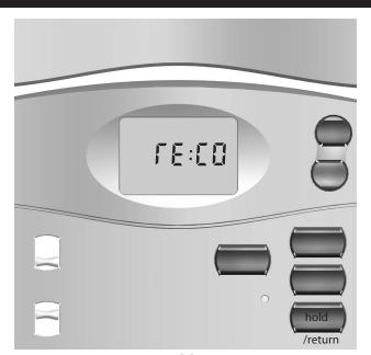
4. Auto recovery – allows heating and cooling systems to gradually recover from an energy-saving setpoint temperature to a comfort setpoint temperature. Auto recovery calculates the time needed to adjust the temperature to the next program setting. When the thermostat is in Auto Recovery mode, the display will flash alternating messages of RECO and the time. Auto Recovery can be disabled by sliding the recovery switch on the back of the circuit board to the disable position.
