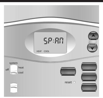
Span setting mode – allows you to adjust the system ON/OFF cycle rate. The default setting is 2 (the system cycles ON or OFF when the temperature is within 1° F (0.5° C) above and below the set temperature.) The span setting can be adjusted if your system is cycling too fast or too slowly.
