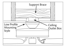
**Low Profile Mounting** fits close to the ceiling, recommended for ceilings less than 8 feet high
