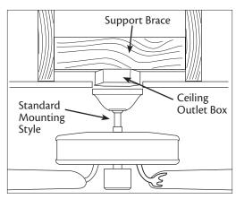
**Standard Mounting** hangs from the ceiling by a downrod (included).
