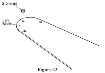
NOTE: Grommets are usually assembled by hand. If you use a tool, make certain you do not damage the grommet or blade when inserting the grommets.
