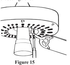
7. Line up the other hole on the motor and fasten the second screw.
