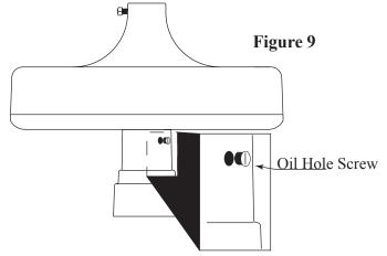
3. Cut the tip off the tube, tilt the fan motor as shown and place the tube into the oil hole of the switch housing. See Figure 10.
