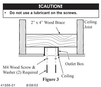
2. Drill two (2) 1/4" diameter holes 2-9/16" apart through the back of the outlet box into the cross brace. There may be two holes at the correct spacing, but they will probably have to be enlarged.
