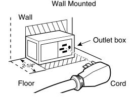
Recommended acceptable electrical outlet area. Orient the electrical receptacle so the length is parallel to the floor.
