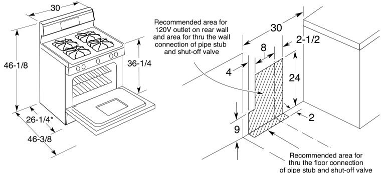
**Installation Information:** Before installing, consult installation instructions packed with product for current dimensional data.
