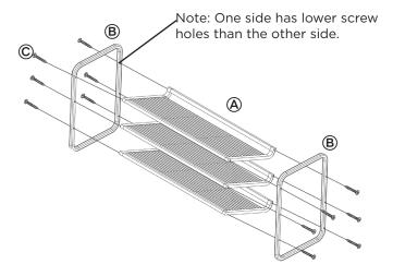
Align everything as shown above. In order for shelves to be slanted, the curved lip needs to be attached to the side with the lower screw holes. Use a hex wrench to tighten each of the 12 hex head screws into place.
