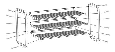
Align everything as shown above. Use a hex wrench to tighten each of the 12 hex head screws into place.
