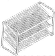
**Alternate assembly:** This assembly shows shelves flat. In order for shelves to be flat, the curved lip needs to be attached to the side with the higher screw holes.
