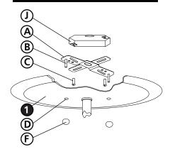
\*\*\* The construction of this fixture will be accomplished by first mounting the mounting stap to the juntion lox, making all neessary electrical connections, harging the fixture from the ceiling, and then installing the glass.
