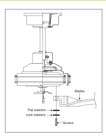
Fasten blade to motor with provided flat washers, lock washers and blade mounting screws. Repeat procedure for remaining blades. Make sure screws are TIGHT! Loose motor screws can contribute to unnecessary hum during operation.
