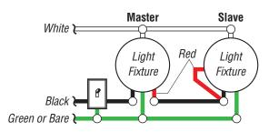
WIRING MOTION SENSING LIGHT TO CONTROL ANOTHER MOTION SENSING LIGHT
