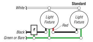
WIRING MOTION SENSING LIGHT TO CONTROL STANDARD FIXTURE
