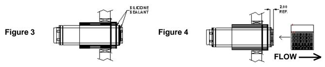
4. The vent section must protrude at least 2 inches into the screened area beyond the end plate of the Wall Termination Assembly (Figure 4). Attach the screen cover using stainless screws. Align the hole in the top (solid) portion of the screen cover with the top of the assembly and securely screw the two pieces together. The screen cover may be easily removed for inspection of the venting system.
