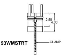
130 Industrial Boulevard • Turners Falls, MA 01376 Phone 800 772 0739 • Fax 413 863 4803 • www.heat-fab.com 4" Adapters — Adapters for appliances with 4" flue collars.
