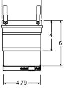
9501NOR P-K Mach Adapter — This adapter is specially designed to connect directly to the vent outlet of P-K Mach Boilers, Series C-300,
