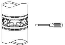
5. Center the Coupler Band around the completed joint and tighten the 7/16" nuts with a hollow nut driver or deep socket. If the assembly must be weather tight, apply a 1/4" bead of sealant to the inside top edge of the Coupler Band approximately 1 inch down from the edge.
