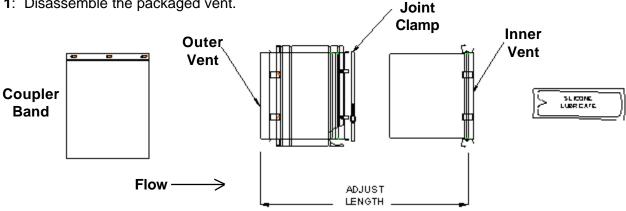
Step 2: Measure edge to edge the distance needed, then add 3 inches total for the joints. The installed length is 13 to 20 inchs for the long adjustable section and 7 to11 inches for the short adjustable section. CAUTION: DO NOT LENGTHEN PAST THE WARNING ARROW.
