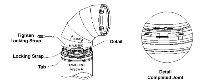
6. Center the Coupler Band around the completed joint and tighten the 7/16" nuts with a hollow nut driver or deep socket. If the assembly must be weather tight, apply a 1/4" bead of sealant to the inside top edge of the Coupler Band approximately 1 inch down from the edge.
