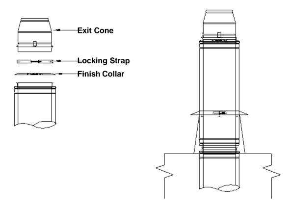
The outlet diameter is typically a 2" reduction in diameter but other sizes may be ordered.
