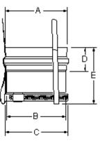
**Raypak Vent Cap Adapter** — This adapter makes the connection between Saf-T Vent products and Raypak's Flue Exhaust Vent Cap.
