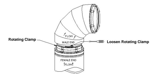
4. Line up the tabs of the rotating clamp with the female end of the preceding vent. Insure the beads on the tabs of the rotating clamp are nested into the groove on the male end. RE-tighten the rotating clamp. If needed use pliers or vice-grips to squeeze together the tabs so they will accept the slots in the locking strap.
