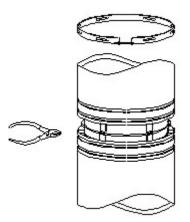
4. Position the Locking Strap slots over the Tabs, making sure each slot encompasses both Tabs. Tighten the Locking Strap with a 7/16" hollow nut driver or deep socket, take caution not to over tighten the clamp causing the vent to collapse.
