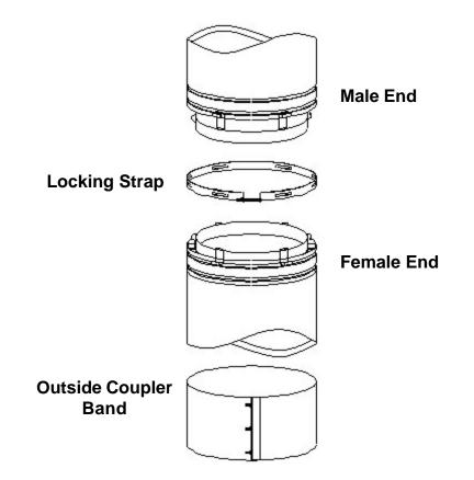
2. Wipe the male and female ends clean with alcohol wipes. On diameter sizes **without** the gasket, at 3/4" from the edge, apply a 1/4" thick continuous, straight-line bead of high temperature sealant to the inside circumference of the female end. Do not use a zig-zag pattern when applying sealant. Smooth down the bead with a flat instrument or your moistened finger.
