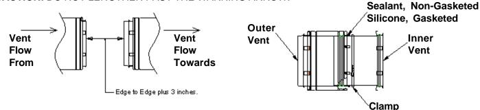
Step 3: Gasketed: Lightly apply the silicone lubricant to the upper ridges of both gaskets in the outer vent. Slide the Inner Vent into the Outer Vent to the desired overall length. Non-Gasketed: Slide the Inner Vent into the Outer Vent to the desired overall length. Apply a 1/4" bead of RTV sealant into the crevice, completely around the vent. Smooth sealant into place.
