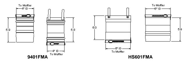
Noritz Adapter — This adapter makes the connection between Saf-T Vent products and Noritz water heaters that require 5" diameter vent.
