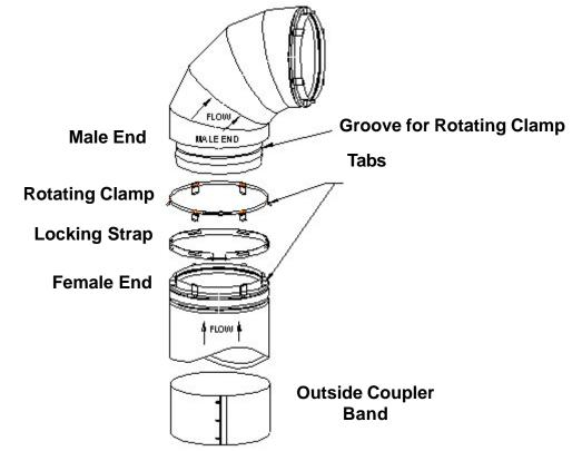
2. Wipe the male and female ends clean with alcohol wipes. On diameter sizes **without** the gasket, at 3/4" from the edge, apply a 1/4" thick continuous, straight-line bead of high temperature sealant to the inside circumference of the female end. Do not use a zig-zag pattern when applying sealant. Smooth down the bead with a flat instrument or your moistened finger.
