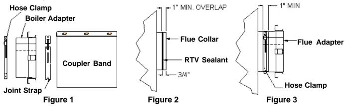
2. All joint surfaces **must** be cleaned with alcohol wipes before applying sealant. Apply 1/4" thick bead of RTV sealant around the outside of flue collar approximately 3/4" from the edge, *figure 2*. Place the adapter over boiler collar lining up the edge of the adapter to the scribe marks, then tighten the hose clamp snugly, *figure 3*. On horizontal flue collars, the split side of the boiler adapter should be installed along the top of the flue collar.
