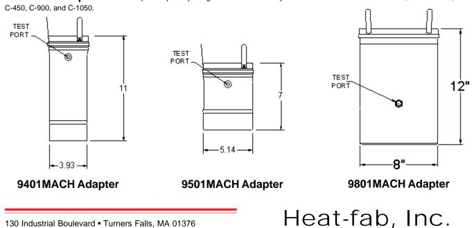
**Raypak Boiler Adapter** — This adapter is specially designed to connect directly into the vent outlet of Raypak's ADB or High Delta boilers. The hose clamp is tightened around the outside of the flue collar to create a mechanical joint.
