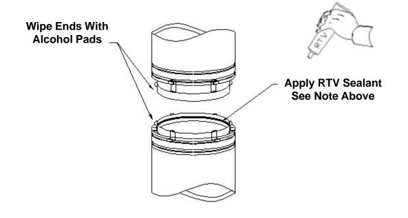
3. Insert the male end into the female end, lining up the Locking Tabs at the same time. If needed, use pliers or vice grips to squeeze together the Tabs so they will accept the slots in the Locking Strap. When assembling elbows and tees, the male end tabs will rotate around the vent to accommodate offsets and direction changes, refer to rotating clamp installation instructions.
