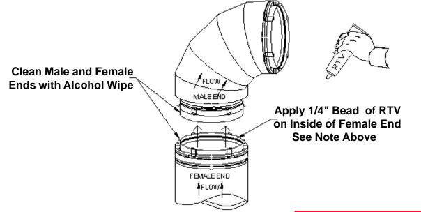
3. Insert the male end into the female end of the preceding vent piece, loosen the rotating clamp on the male end of the fitting with a 5/16" nut driver.
