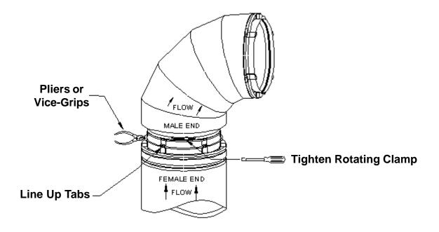
5. Position the Locking Strap slots over the Tabs, making sure each slot encompasses both Tabs. Tighten the Locking Strap with a 7/16" hollow nut driver or deep socket. **CAUTION**: DO NOT over tighten the clamp, as it may cause the vent to collapse.
