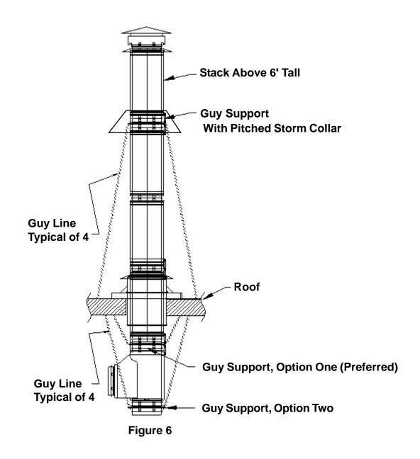
**Note**: When installing above the roof use a "pitched storm collar", part # IP-\_\_SC3 to prevent rain water from entering the outer wall of the vent and running down the stack.
