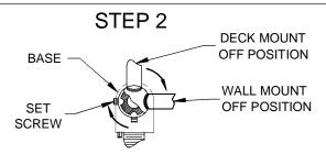
NOTE DEPTH OF SET SCREW PRIOR TO LOOSENING.
