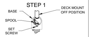
UNIT IS SHIPPED IN DECK MOUNT CONFIGURATION. TO CONVERT TO WALL MOUNT CONFIGURATION, POSITION ARM IN "DECK MOUNT OFF POSITION" AS ABOVE.
