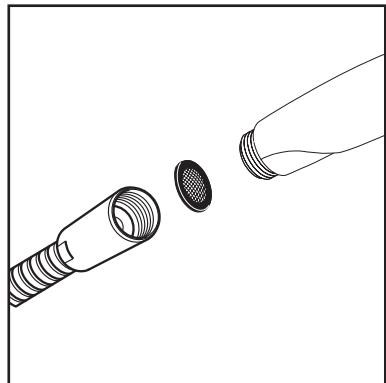
If the flow of water becomes noticeably less, remove and clean the screen washer.
