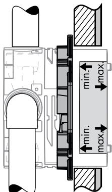
Install the valve so that the outside surface of the finished wall falls between the "min" and "max" markings.
