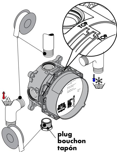
If an outlet is not to be used, seal it with a  $\frac{3}{4}$ " plug (included).
