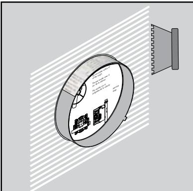
Spread waterproof adhesive (not included) on the backing board around the iBox.
