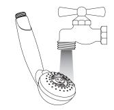
Reinstall the handshower. Turn on the water and allow the handshower to flush for at least one minute.
