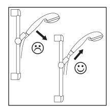
To move the slider up and down the bar, loosen the slider knob. Move the slider to the desired position. Tighten the knob.
