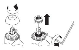
Replace the high temperature limit stop so that the pin on the cartridge is in the desired slot on the limit stop. Note: the temperatures given in the diagram assume a water heater temperature of 140° F, a cold water temperature of 50° F and a water pressure of 45 PSI.
