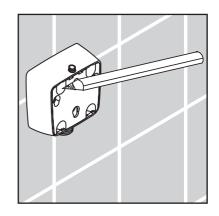
Drill the holes with a 6 mm bit. Use extreme caution - do not drill into the water line.
