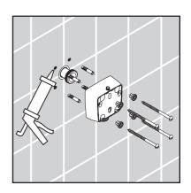
Remove the long bottom mounting screw on the Allrounder. Replace with the shorter screw included with the adapter.
