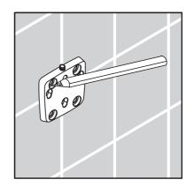
Put the mounting plate away in a safe location. Drill the holes, using a 6 mm bit.
