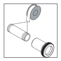
Screw the test nipple / mounting piece assembly into the drop-eared ell.
