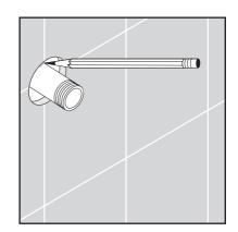
Measure the test nipple to the mark.
