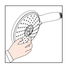
Remove scale deposits on the spray face by using a commercial limescale remover such as Lime-Away<sup>TM</sup> or  $CLR^{TM}$ . Follow the label instructions carefully. Soak only the spray face.
