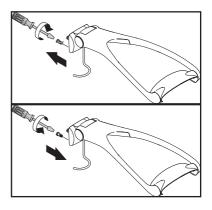
Attach the Allrounder to the mounting plate. Tighten the set screw.
