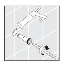
Position the mounting plate over the mounting piece. Use a grease pencil or similar tool to mark the position of the screw holes.
