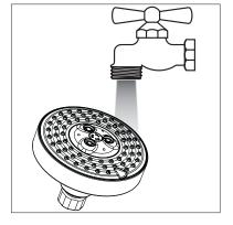
Reinstall the showerhead. Turn on the water and allow the showerhead to flush for at least one minute.
