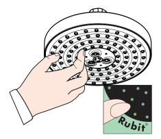
If scale deposits are noticed on the spray face, pour about 3/4" of a commercial scale remover, such as Lime-Away™ or CLR™, into a shallow dish. Dilute the remover according to the label instructions.
