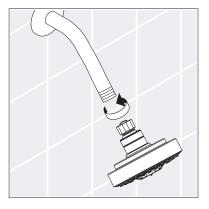
If the flow of water becomes less over time, remove and clean the filter gasket.
