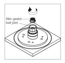
Carefully install the showerhead on the shower arm. Because of the self-sealing filter gasket, Teflon tape is normally not required.
