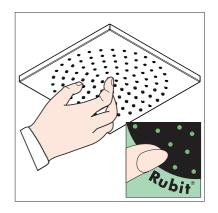
If scale deposits are noticed on the spray face, pour about 3/4" of a commercial scale remover, such as Lime-Away<sup>TM</sup> or  $CLR^{TM}$ , into a shallow dish. Dilute the remover according to the label instructions.
