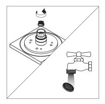
The showerhead incorporates the Rubit™ cleaning system. If scale deposits are noticed in the spray channels, turn the water on lightly and rub the spray channels with a finger or a sponge.
