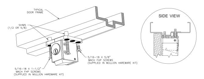
**NOTE:** The shims are to be used when the top fitting overhangs the stop.
