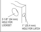
Drill 2-1/8" (54 mm) hole through door face as marked for lockset. (It is recommended that holes be drilled from both sides on wood doors to prevent splitting.) Drill 1" (25.4 mm) hole in center of door edge for latch.
