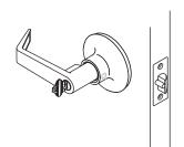
B. Using catch release tool, press the lever catch and pull the lever off.
