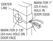
MARK FOR 1" Measure center line of lock; height as (25.4 mm)
