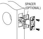
C. Insert latch and tighten screws. NOTE: Latchbolt bevel must face to closing direction. For doors with a 1-1/8" wide latch cutout, insert latch through optional spacer and then install latch in door.
