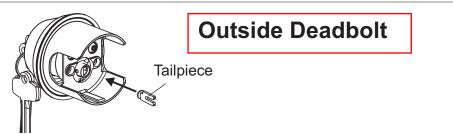
Load the tailpiece in the vertical direction and turn 90 degrees to horizontal position.
