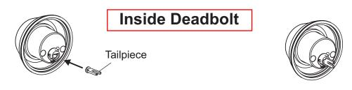
Load the tailpiece in the horizontal direction and turn 90 degrees to vertical position.
