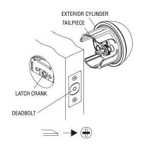
B. Press exterior cylinder flush against door. Install interior tail piece vertically through latch crank. Press interior cylinder flush against door and tighten mounting screws.
