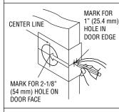
Measure center line of lock; height as desired from finished floor. Select 2-3/4" or optional 2-3/8" backset, fold and apply template to high side of bevel door and mark center of door edge as indicated on template. Mark center hole on door face through guide on template.
