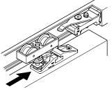
**1. From the side** Fixed pocket cover doesn't have to be removed Cover plate above opening has to be removable
