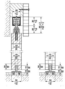
The two-way suspension bracket allows the door leaf to be hung and to be taken off in two different ways:
