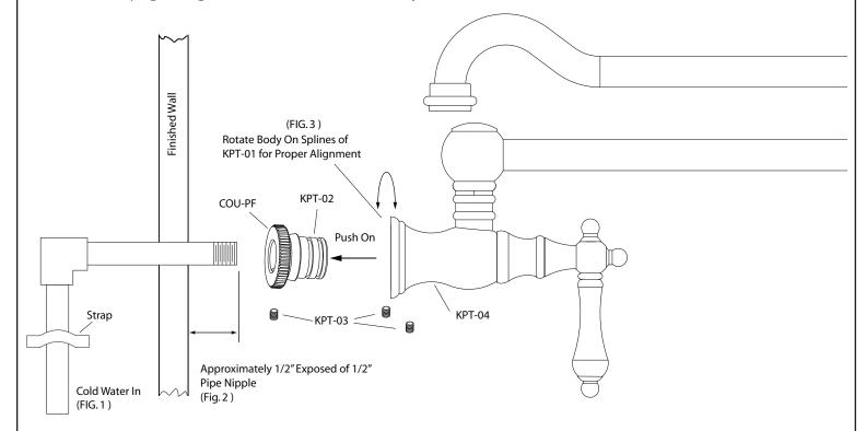
**Step 5**- Rotate faucet until correct alignment is made (spout should be pointing straight down) Fig. 3. Push the faucet body onto the quick connector over the two o-ring seals **KPT-02**. The splines inside the faucet body should line up with the splines on the quick connector.
