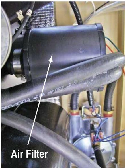
**Figure 4.7 — 8kW Engine Air Cleaner Location**
