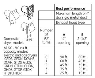
For every extra 90° elbow, reduce the allowable vent system length by 10 ft.
