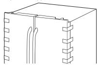
Start with left-hand door first: Remove the hinge cover on top of the left refrigerator door by removing all hex screws and pulling it up. Do the same for the right-hand door and the middle cover.
