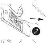
Remove the replacement filter from the plastic. Insert the filter into the housing by pushing it in. The filter will snap into place.
