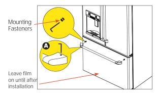
Reinstall the handles using the same procedure as removing.
