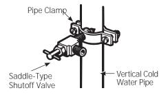
NOTE: Commonwealth of Massachusetts Plumbing Codes 248CMR shall be adhered to. Saddle valves are illegal and use is not permitted in Massachusetts. Consult with your licensed plumber.
