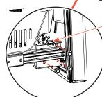
Align and insert tab on freezer door bracket into slot on freezer slide bracket.
