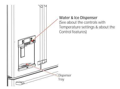
If no water is dispensed when the refrigerator is first installed, there may be air in the water line system. Press the dispenser paddle for at least five minutes to remove trapped air from the water line and to fill the water system. To flush out impurities in the water line, throw away the first six full glasses of water.
