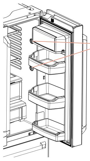
There is LED lighting in fresh food compartment and on the bottom of the fresh food doors to light the freezer compartment.
