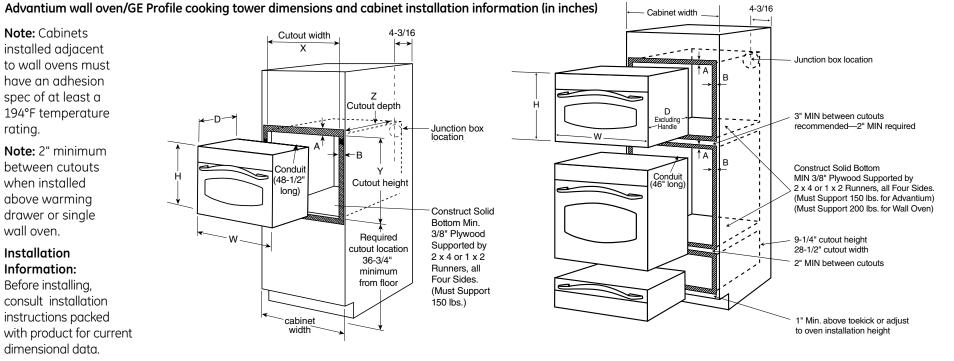
A=Allow 1" overlap of oven over top and bottom edges of cutout. B=Allow 11/16"-3/4" for overlap of oven over side edges of cutout. A=Allow 1" overlap of oven over top and bottom edges of cutout. B=Allow 11/16"-3/4" for overlap of oven over side edges of cutout.
