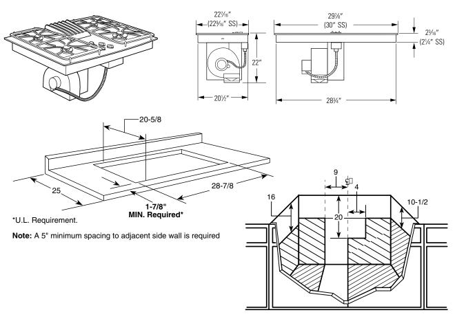
\*Note: A 5" minimum spacing to adjacent side wall is required Dimension and installation information are shown in inches.
