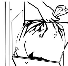
As is true of most appliances, proper care is needed to give you continued satisfaction. Before cleaning the compactor, turn the knob to the **OFF** position and remove it. If you will be away for more than a couple of days, remove the compactor bag. Lock the compactor by removing the knob and store it in a safe place.
