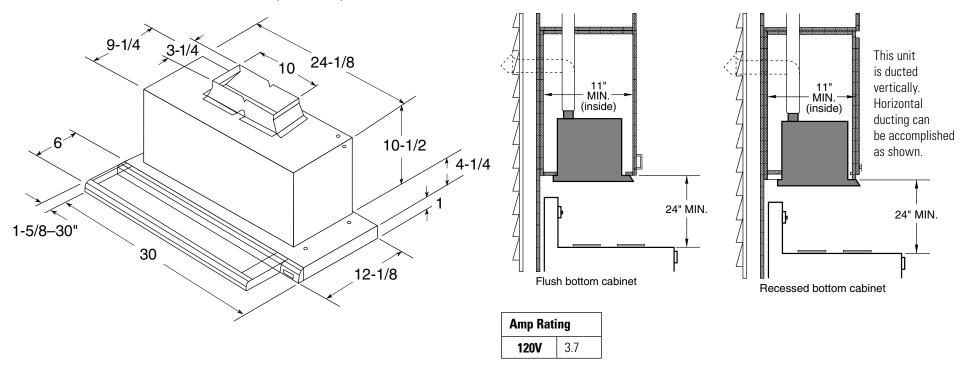
**Note:** Remove glass visor from unit before installing hood in cabinet to protect visor from damage.
