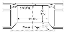
Side-by-Side Units in Under-Counter Installation
