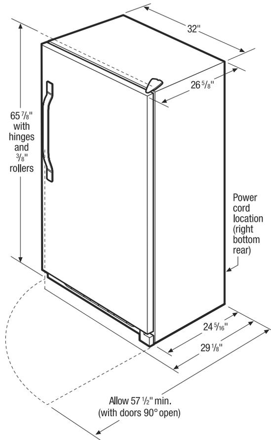
\* When installing refrigerator adjacent to wall, cabinet or other appliance that extends beyond front edge of unit, 20" minimum clearance recommended to allow for optimum 140° door swing, providing complete basket access and removal. (Absolute 3" minimum clearance will ONLY allow for 90° door swing which will provide limited basket access with restricted removal.)
