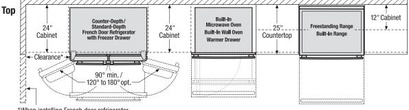
\*When installing French door refrigerator adjacent to wall, cabinet or another appliance that extends beyond front edge of unit, 20" minimum clearance recommended to allow for optimum 120° to 180° door swing, providing complete drawer/crisper access and removal. (Absolute 4-1/2" minimum clearance will ONLY allow for 90° door swing which will provide limited drawer/crisper access with restricted removal.)
