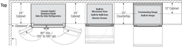
\*When installing side-by-side refrigerator adjacent to wall, cabinet or another appliance that extends beyond front edge of unit, 20" minimum clearance recommended to allow for optimum 120° to 180° door swing. providing complete drawer/crisper access and removal. (Absolute 4-1/2" minimum clearance will ONLY allow for 90° door swing which will provide limited drawer/crisper access with restricted removal.)
