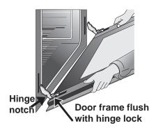
Figure 36: Replacement and location of hinge arm and roller pin
