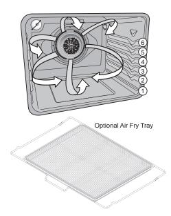
Figure 24: Optional Frigidaire Air Fry Tray. Use rack position 4 with tray or dark pan with low or no sides for best results.
