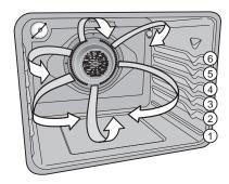
Figure 17: Oven rack positions
