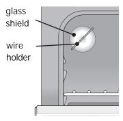
Figure 37: Oven light protected by glass shield
