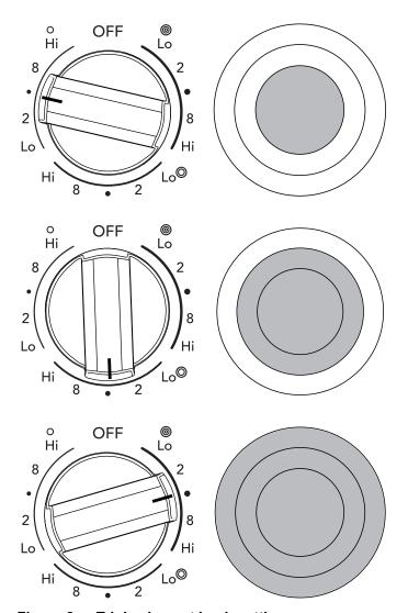
Figure 8: Triple element knob settings
